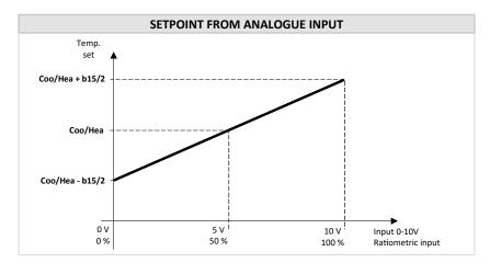
Correction calculation with ratiometric input (b20=1):
