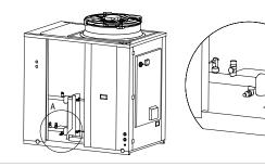
If the unit must be completely drained, first close the manual inlet and outlet shutters (not supplied) and then disconnect the pipes on the water inlet and outlet so that the liquid in the unit can drain (to make this operation easier, it is advisable to install two external drain cocks between the unit and the manual shutters on the water inlet and outlet).
