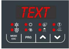
It is used to select the operating mode, and to reset the manual resetting alarms. The operating mode changes as per the sequence below each time you press the Mode button:
